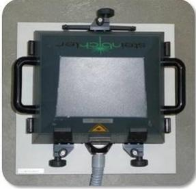
Detection of artificially induced defects on backside with ISISmobile 3100
